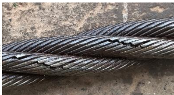
Elements are cut due to bending fatigue
