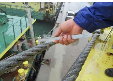
Wire rope inspection
